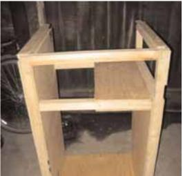
Front wall is sheathed to hide the polystyrene. Bottom stop for the baffle is installed at the lower end of the baffle rails.
