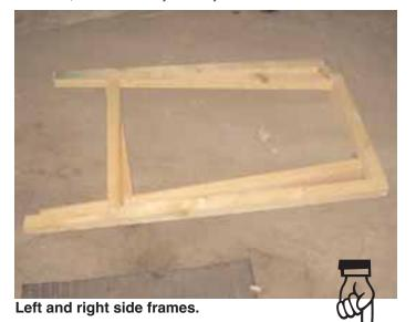
Sides are attached to the back wall. Slider rails for front baffle are attached to front edge of side walls.
