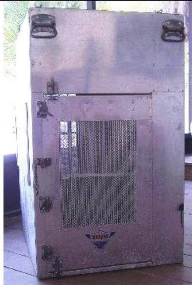
For larger monkeys and apes, a strong but lightweight aluminum crate such as this Airborne is good. Notice there are 6 different locks on this door. These crates are riveted construction, much like an airplane. The one pictured measures 42" high, 33" deep, 25" wide. A full service welder may be able to make one for you.
